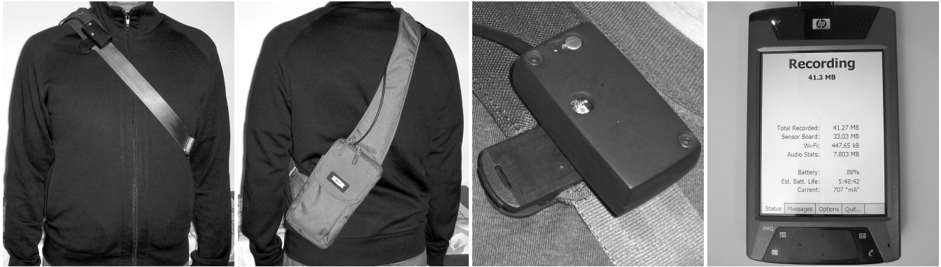
(a) Front: MSB is on right shoulder (b) Back: PDA is in bag. (c) MSB. Microphone is at top. (d) PDA and data collection program.
